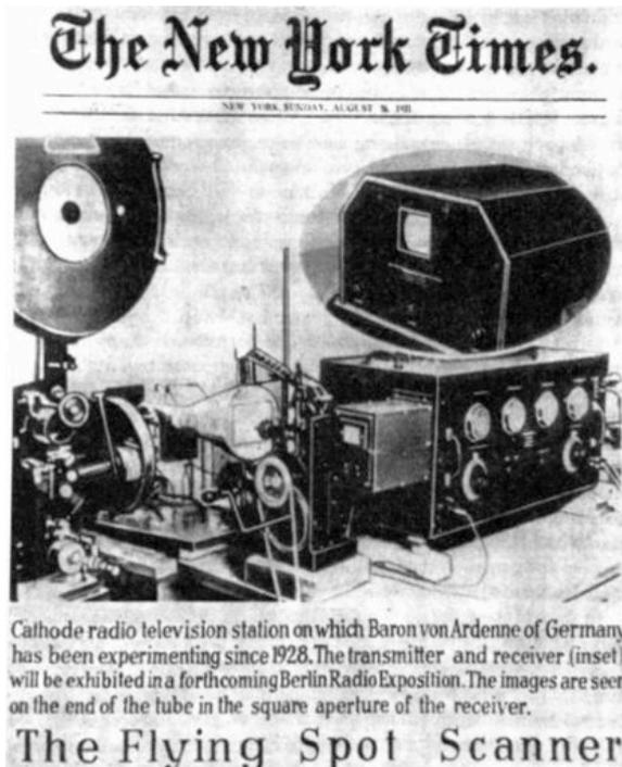
At the end of the 19<sup>th</sup> century the German physician Ferdinand Braun succeeds in the path-breaking development of the so-called cathode ray tube, which enables the magnetic control of light-points, out of which images are to be generated.
